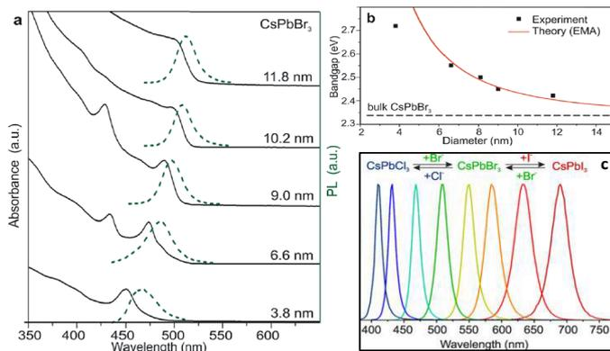
**Figure 1:** a) Quantum confinement effect observed in the absorption and emission spectra of  $\text{CsPbBr}_3$  QDs.[4] b) Experimental and theoretical (effective mass approximation, EMA) dependence of the band gap energy from the QD size. c) Normalized PL spectra of 10-nm  $\text{CsPbX}_3$  QDs with varying halide composition.[5]
